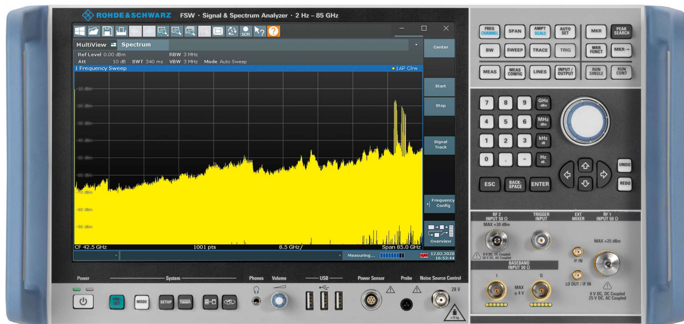
Fig. 3: The R&S®FSW85 covers the entire spectrum in a single sweep with preselection from 2 Hz to 85 GHz. The 4 GHz radar signal in the E band at 79 GHz is clearly visible.
