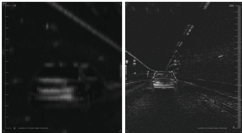
Fig. 5: This simulation gives an impression of the difference between an imaging radar and a conventional automotive radar. Its resolution is so high that it can detect and separate objects that are close together, such as a pedestrian next to a cyclist, and process their individual 4D coordinates.
