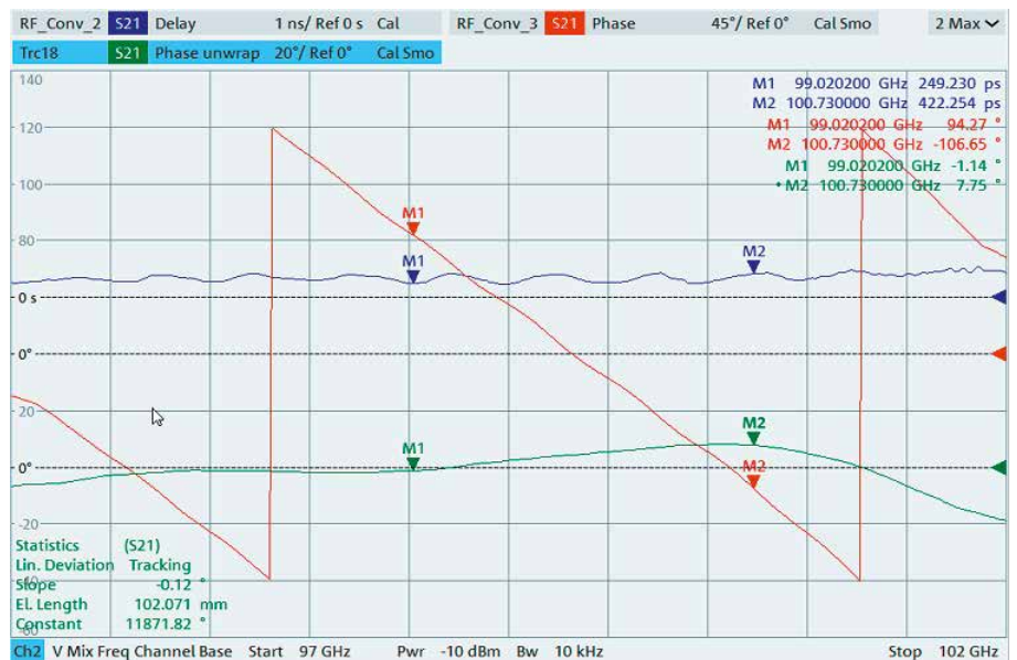
Fig. 3: Phase (red), deviation from linear phase (green) and group delay (blue) of the mixer under test.
