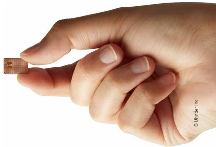
Fig. 4: It is hard to believe that this small chip is a complete multi-channel radar with all signal processing circuitry. All that is missing are the antennas.
