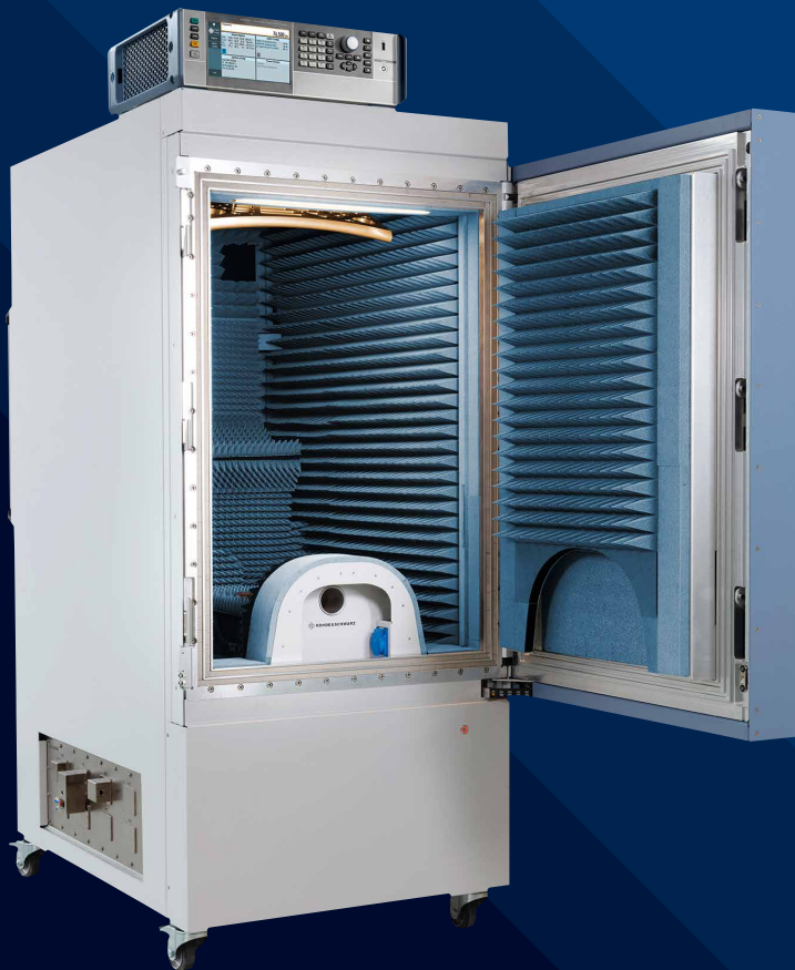
Fig. 3: The test solution for automotive radar sensors, consisting of the R&S®ATS 1500C shielded test chamber and the R&S®AREG100A radar echo generator. For operation, the remotely controlled echo generator is mounted on the rear wall of the chamber.
